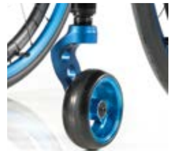
// NTR080008 Castor fork, aluminum, one-arm, blue
