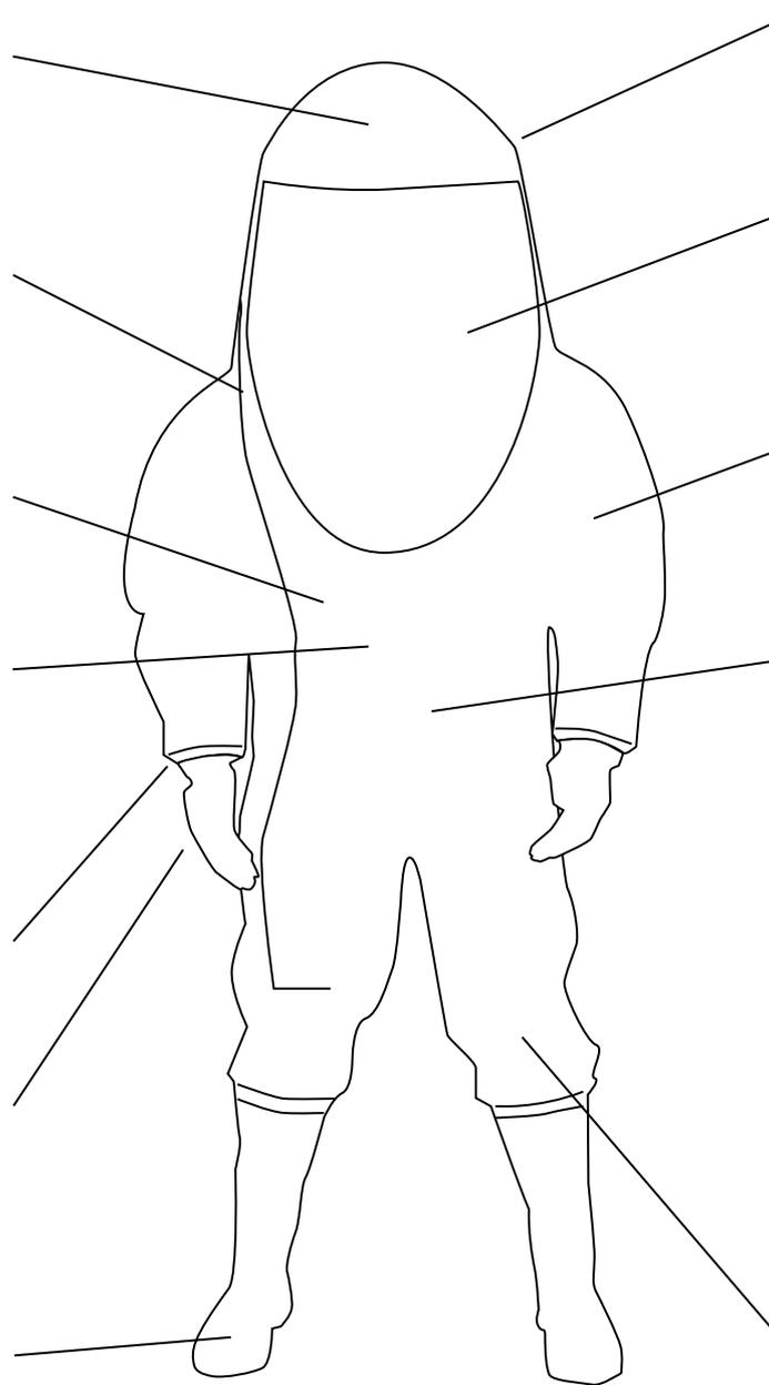
**Two exhalation valves** maintain a comfortable working pressure inside the suit
